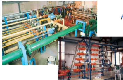
View and principle of the primary nozzle calibration bench "pisc"
