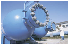
High pressure tanks 200 bar
